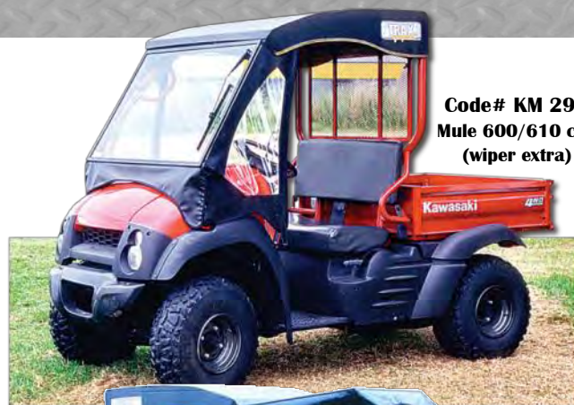
← Windscreen hinges for toolbox access, supported by gas struts
