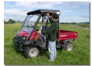
PVC dome on side fenders can easily be taken off or re attached.
